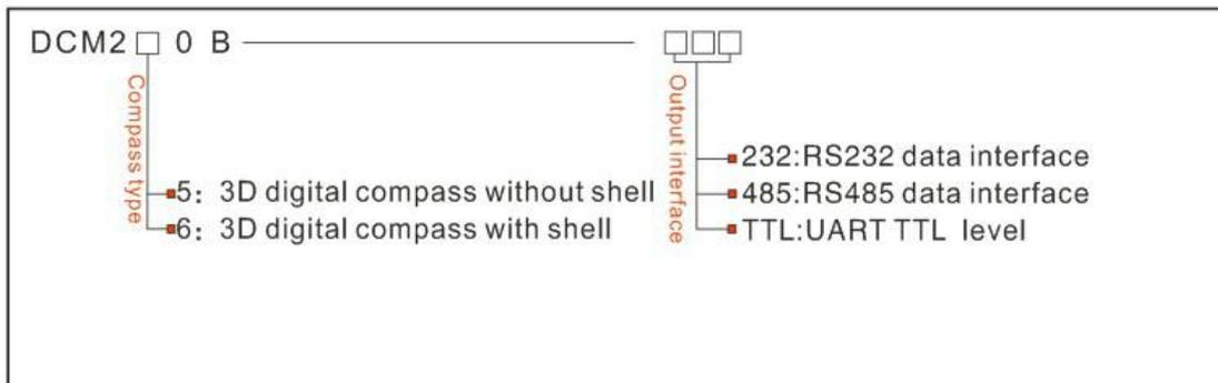
E.g: DCM260B-232: 3D with enclosure sealed/RS232 output
